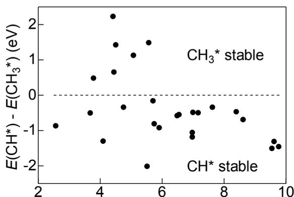
Figure 2. Energy difference between CH\* and CH<sub>3</sub>\* on the stable surface of 26 binary alloys.
